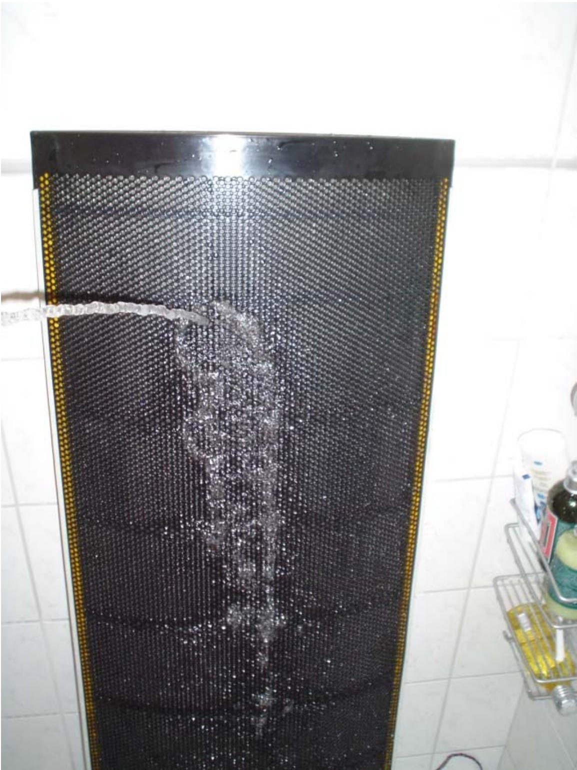
12. Once the washing of the panel was completed, I lifted the panel and shook it up and down, a lot of the water inside the Stator will come out.
